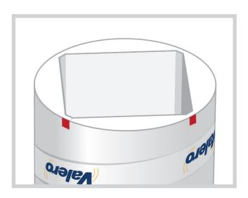
When setting out the pillar, mark the square section first on the ground. Then, mark the screenings of the pillar faces on the formwork and matched to the wrought marks.
